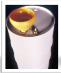
Waste drum with disposal funnel
